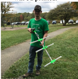
Stephen posing with his fox antenna, much of which was 3d printed.
